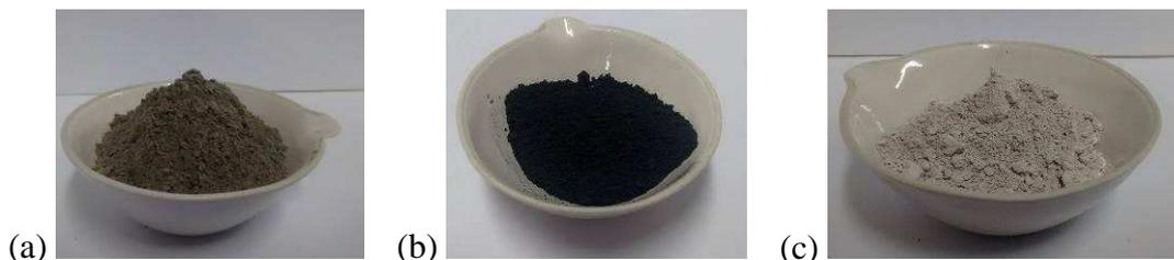
Figura 9. Amostras peneiradas (a) clínquer; (b) dregs e (c) grits.
