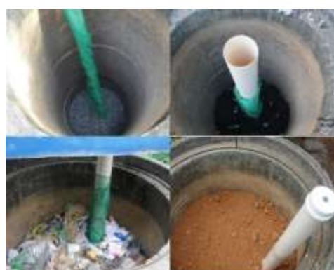
Figure 2. Filling the experimental unit U1 ( grits and dregs and MSW)
